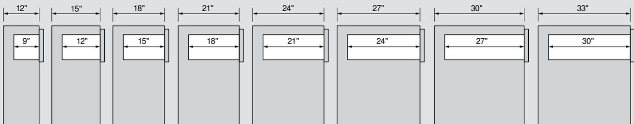
TANDEM series runners are based on the American standard 3" cabinet depth system, therefore, the runner lengths come in 3" increments. TANDEM plus runners are available for drawers from 9" – 30" in length.
